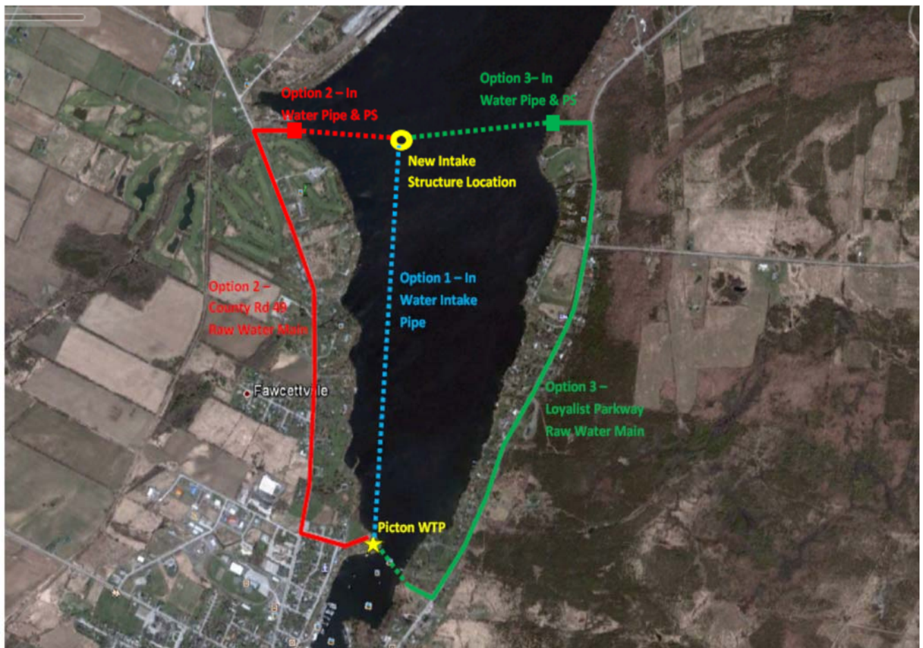
Figure 9.1: Alternative Routing of Intake Pipe from WTP to Preferred Intake Location
